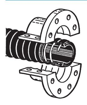
The Bulk-Flex coupling is made of the highest quality cast aluminum. The coupling consists of two halves with internal threads designed to be mechanically attached over the outside of the hose (see illustration below). The Bulk-Flex coupling is designed for a working pressure of 150 PSI. Flange drilling conforms to ANSI 16.5. See page 7 for hose information.
